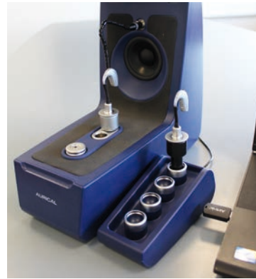
Figure 2. Setup for verifying binaural directionality.
